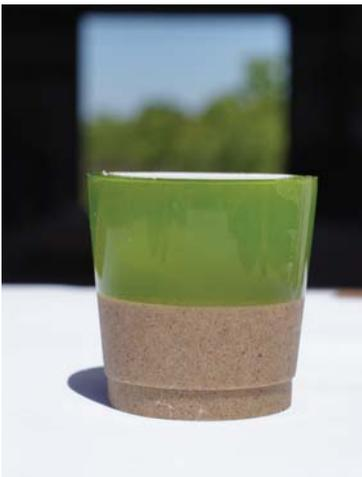
LEFT: Set acrylamide grout sample. The upper half of the sample is pure acrylamide with dye. The lower half of the sample is play sand that has been permeated and solidified with the grout.
