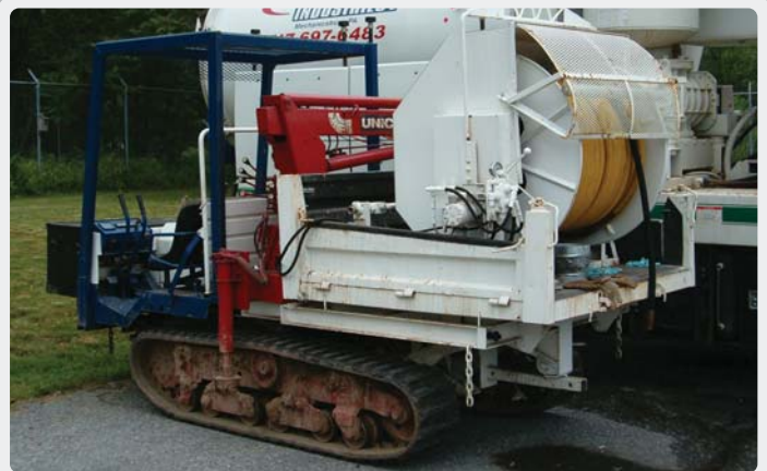
Complete grouting inspection and delivery capability is transported by truck, which carries 500' of delivery hose. When further accessibility by truck becomes prohibitive, an additional 500' of hose is provided via remote grouter unit.
