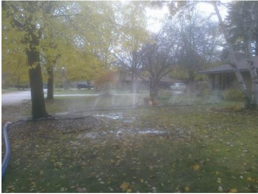
Figure 2. Soaker Hose rain simulation
