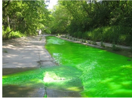
Figure 3. Storm Sewer dye flooding
